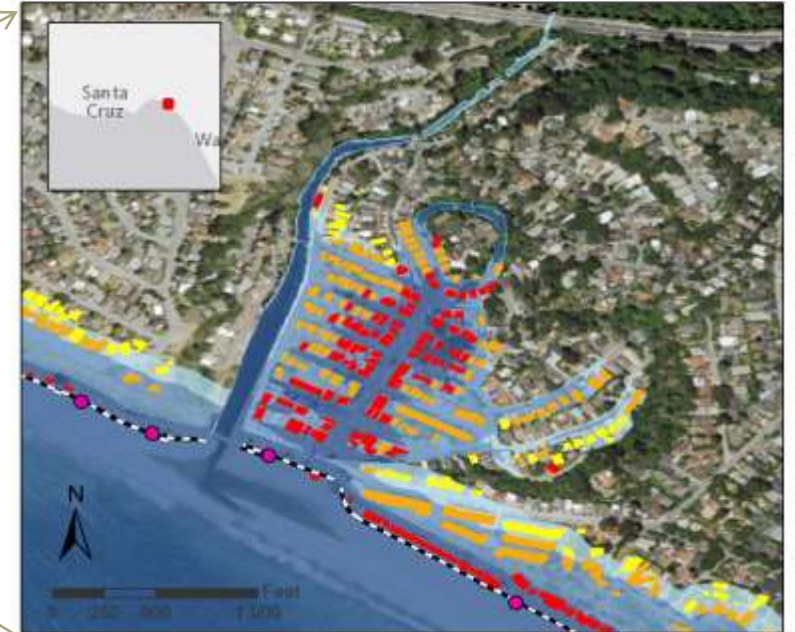
RIO DEL MAR BUILDINGS VULNERABLE TO COASTAL STORM FLOODING
