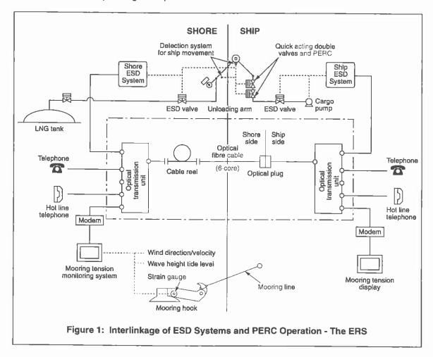
In developing these criteria, the underlying rationale is that the mooring lines must provide secure attachment between ship and shore allowing very little relative movement. This means the hard arms also remain secure and the risk of arm rupture, caused by ship break-out, should not occur. However, although this basic framework underpins safety at the ship/shore interface, it provides only a single defence against risk of spillage and the generation of dangerous gas clouds.
