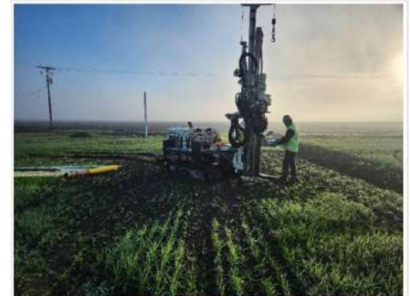
Photograph 2. Example of small drill rig that would be used at site.
