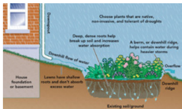
Diagram of a Typical Rain Garden
