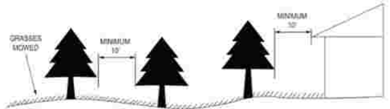
Commentary Figure 603.2.2 10-FOOT SEPARATION BETWEEN TREE CROWNS AND STRUCTURES
