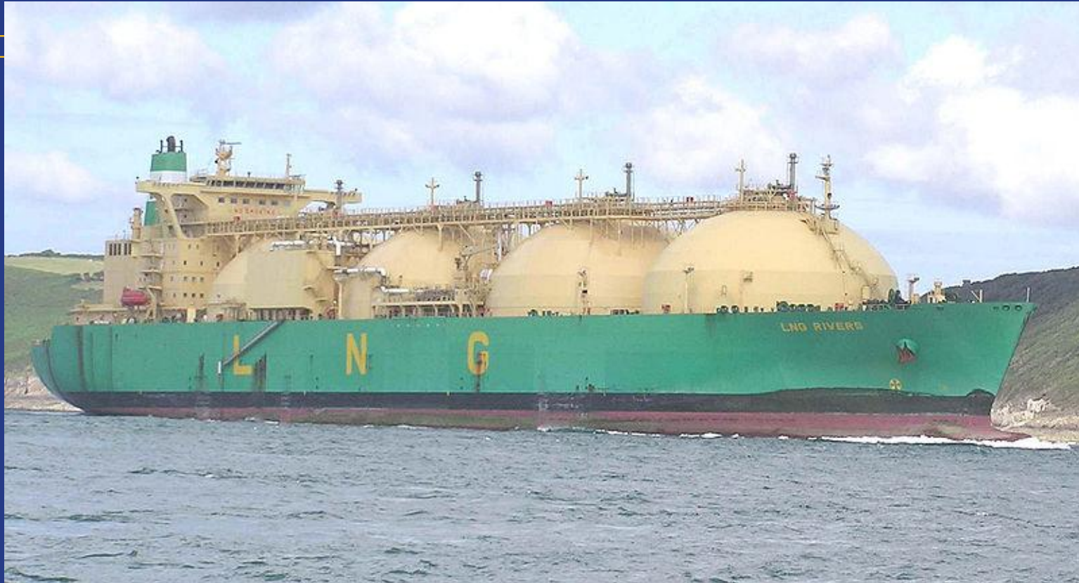
LNG Rivers, a Moss-type carrier with a capacity of 135,000 cubic metres
